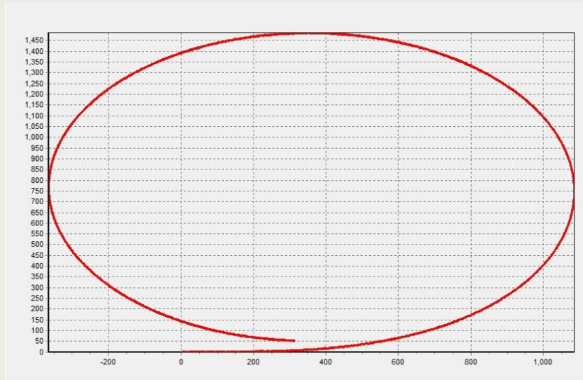
Figure 11 Field sea trial logged data during turning in a full circle (ship course)
